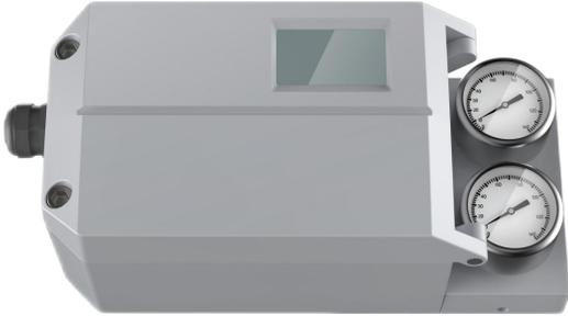
**IP5500 intelligent valve positioner is mounted on pneumatic actuators. It's used to control air intake and exhaust of the pneumatic actuators to drive the valve position to the set point by calculating both data from 4-20mA DC signal and feedback position.**
